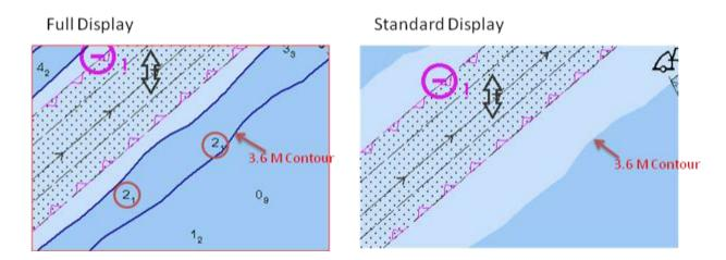
Since the ECDIS does not set off any type of warnings or alarms for these types of soundings in any display mode, it is important that the mariner turn soundings on during route planning and route monitoring to ensure that there are no isolated soundings in the voyage path.
